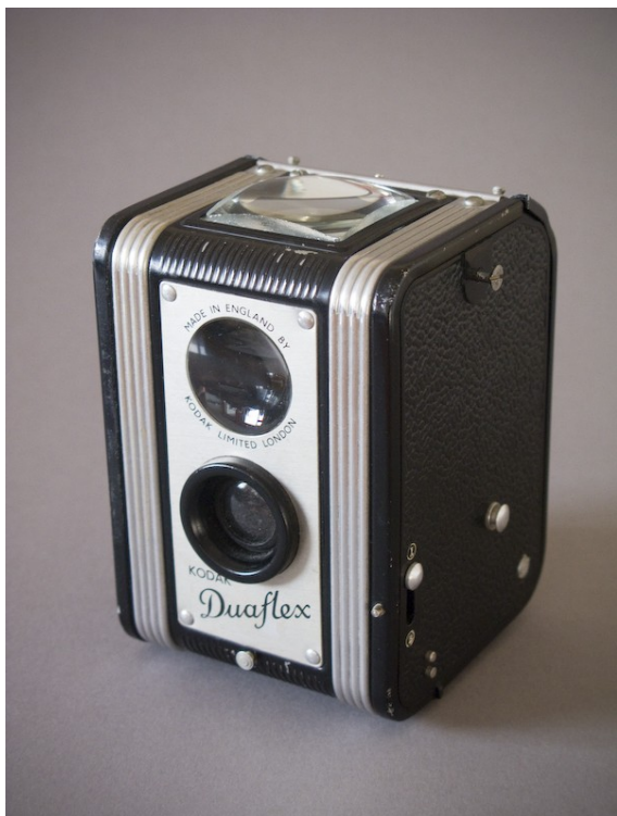
The Kodak Duaflex. This is the first model of the Duaflex, which was available in the UK in the late 1940's and early 1950's. Note the glass bubble viewfinder.
