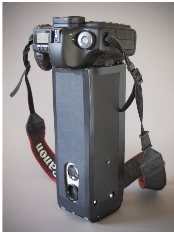
The whole contraption. Duaflex with cardboard snorkel and Canon DSLR, which will photograph the bubble viewfinder.
